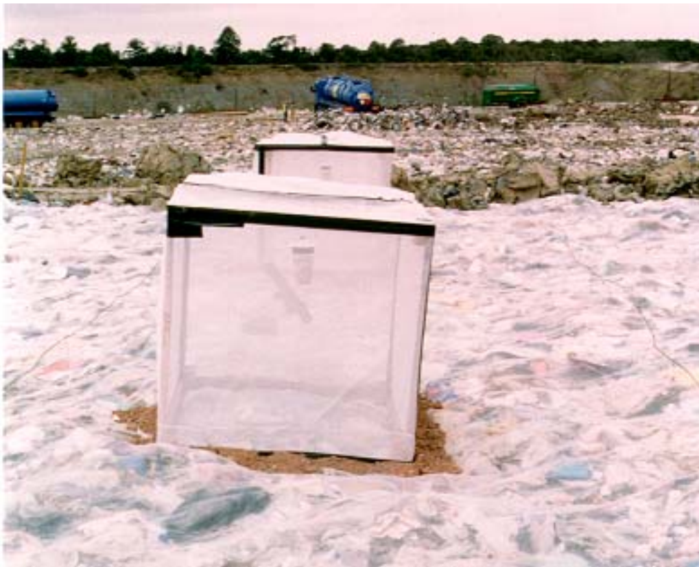
Agralan Enviromesh covered plot showing the fly proof cage with a Victor fly trap suspended from the centre.
