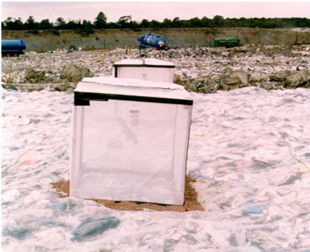
Agralan Environmesh covered plot showing the fly proof cage with Victor fly trap suspended from the centre
